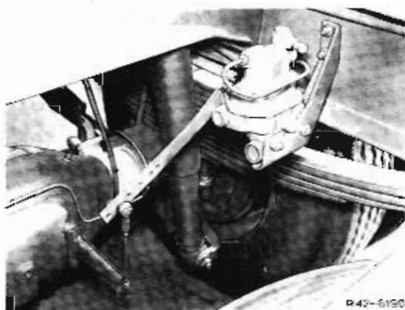
Fig. 3 Automatic brake force regulator on rear axle
